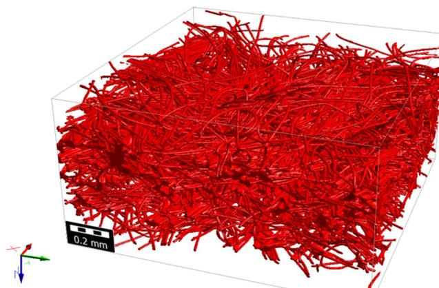
**Figure 2.** Three dimensional of filter material with GeoDict software
