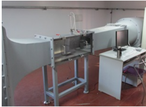
Figure 11. Experiments with the wing models in a low speed wind tunnel 图 11. 低速风洞测试实验
