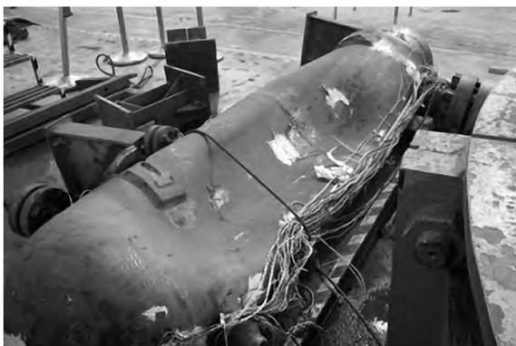
Figure 1. Deformation of pressure vessels under internal pressure
