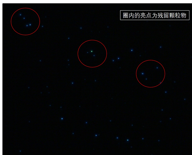
Figure 8. Etched surface morphology after DHF rinse for 2 mins (Microscope dark field)
