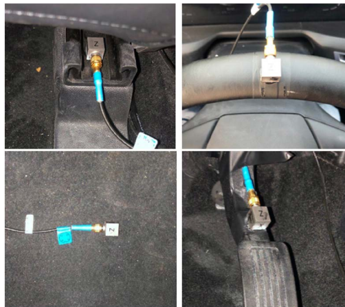
Figure 2. Vibration acceleration test point position
