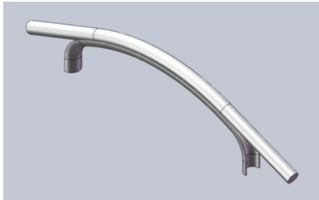
Figure 1. Contact relationship between load-bearing cable and saddle 图 1. 承载索与鞍座接触关系
