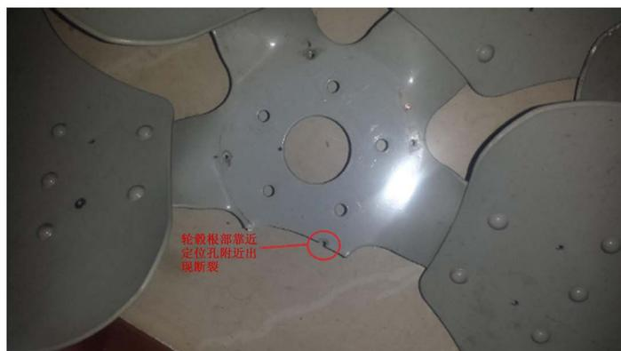
Figure 11. Impeller fracture
