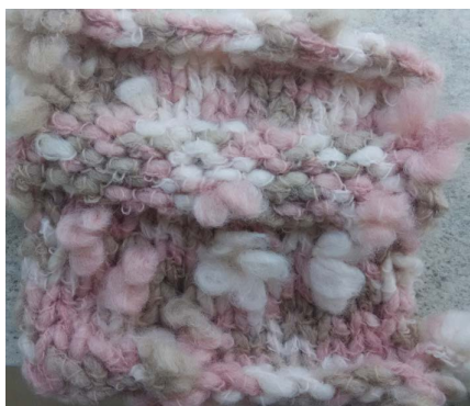
Figure 3. Fabric samples woven with single strands of butterfly yarn 图 3. 单股蝴蝶纱编织而成的面料小样
