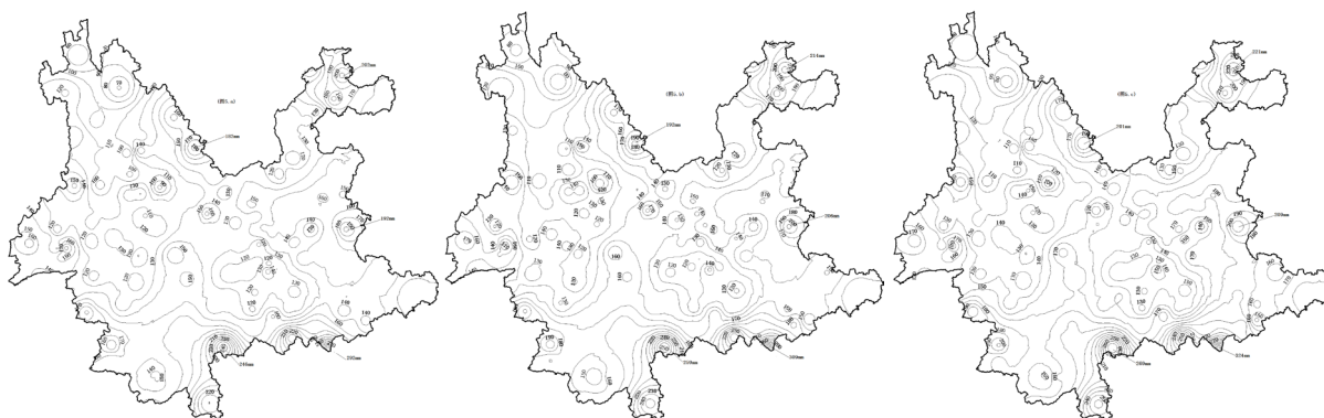
Figure 5. Distribution of extreme maximum daily rainfall in Yunnan in different recurrence periods (100 a (a); 150 a (b); 200 a (c); unit: mm)
