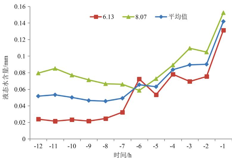
**Figure 2.** The time variation of average liquid water content from 12 h to 1 h before precipitation for individual cases at Xingtai Station (Unit: mm)
