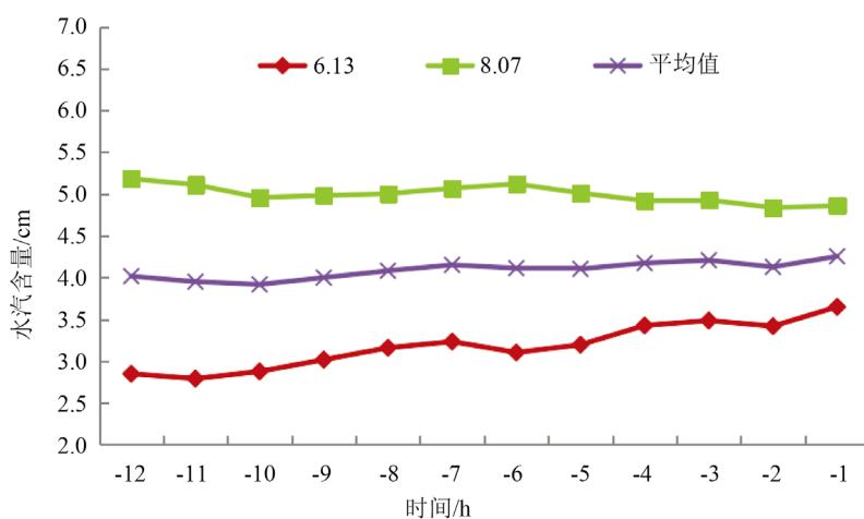
**Figure 1.** The time variation of average water vapor content from 12 h to 1 h before precipitation for individual cases at Xingtai Station (Unit: cm)
