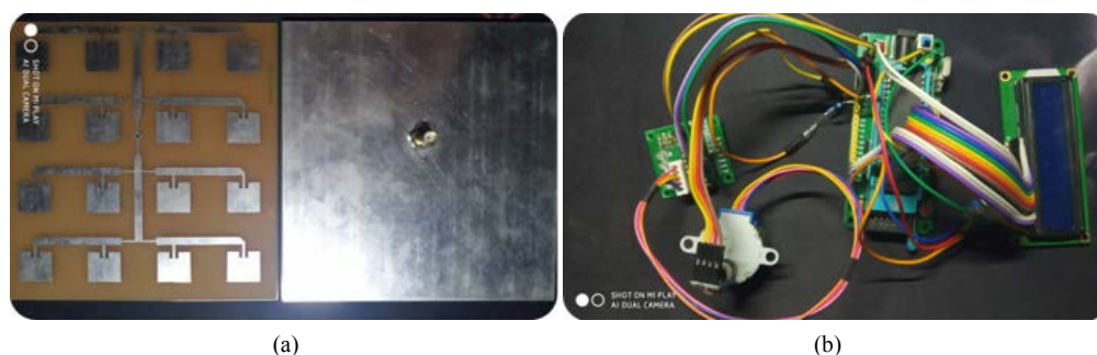
Figure 5. Designed real object. a) Antenna array; b) Intellectual induction system (C51-based) 图 5. 设计实物图。a) 天线阵列; b) 智能感应系统(基于 C51)
