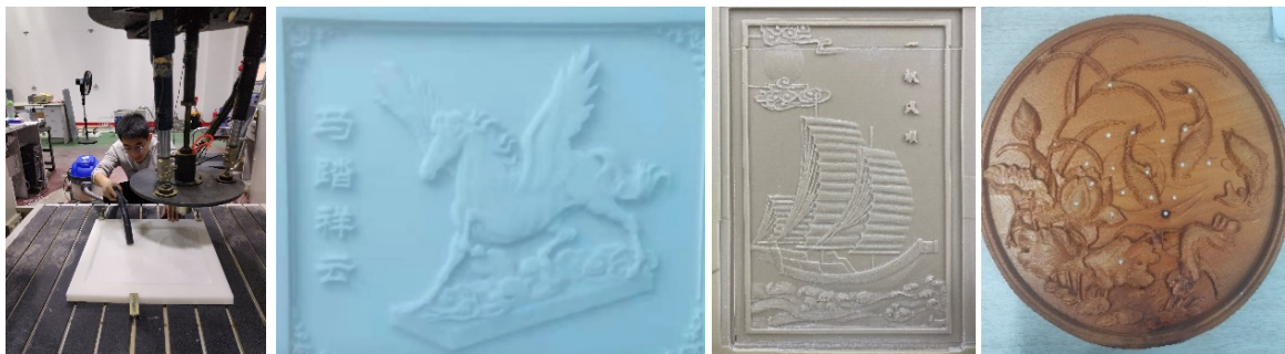
Figure 3. Practical operation and carving works by the new hybrid-robot prototype
