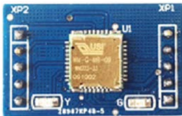
Figure 4. The real figure of The Marvell 88W8686 WIFI module
