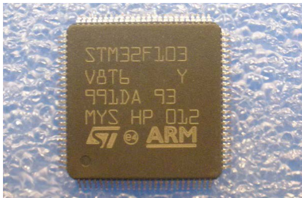
Figure 2. The real figure of STM32F103 图 2. STM32F103 实物图
