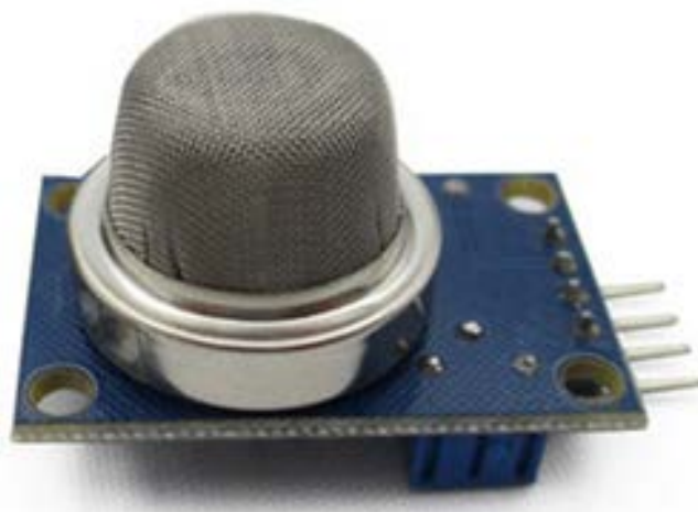
Figure 7. The real figure of The MQ-2 smoke sensor 图 7. MQ-2 烟雾传感器实物图
