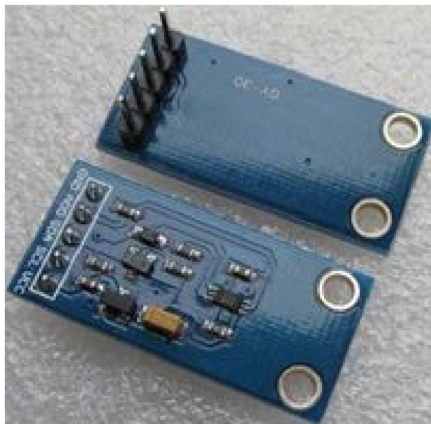
Figure 6. The real figure of BH1750FVI light intensity sensor 图 6. BH1750FVI 光强传感器实物图
