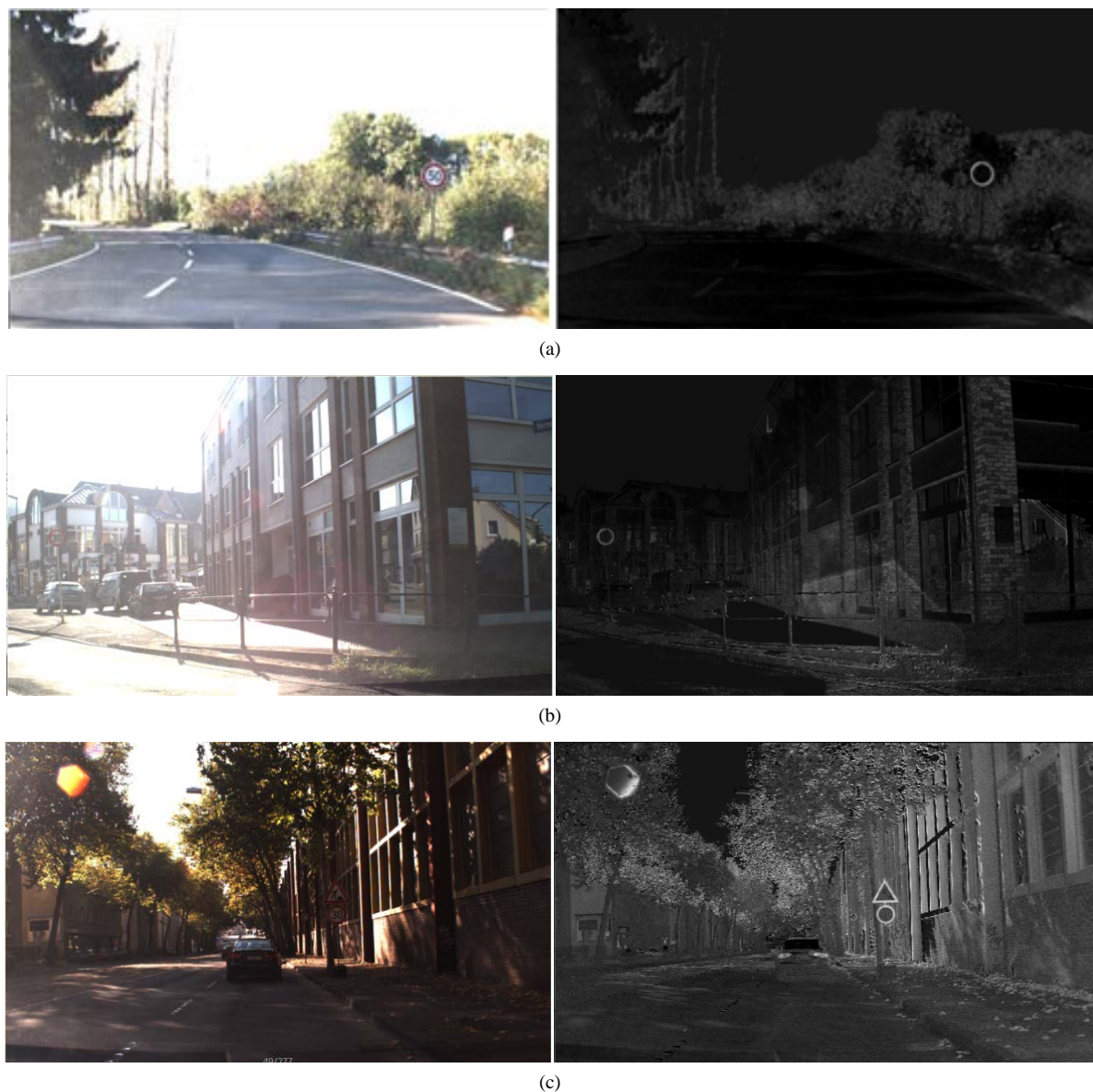
Figure 2. The effect of red-blue processing (a) The image of normal brightness and the effect of red-blue processing; (b) The overexposure image and the effect of red-blue processing; (c) Low light image and the effect of red-blue processing
