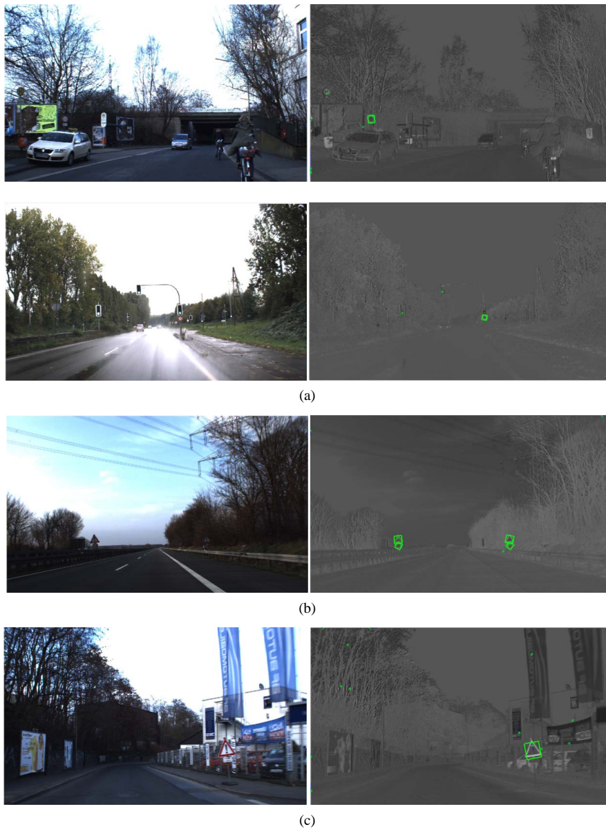
Figure 6. The traffic sign ROI detection results of our method (a) The robustness of our method to geometric scale change; (b) The robustness of our method to contrast change; (c) The robustness of our method to geometric rotation 图 6. 本文方法的交通标志 ROI 检测结果 (a) 本文方法对几何尺度变化的鲁棒性; (b) 本文方法对对比度变化的鲁棒性; (c) 本文方法对几何旋转的鲁棒性
