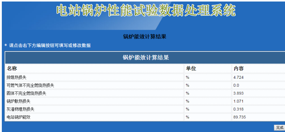
Figure 7. Data processing system for performance test of power plant boiler-results page of boiler energy efficiency calculation
