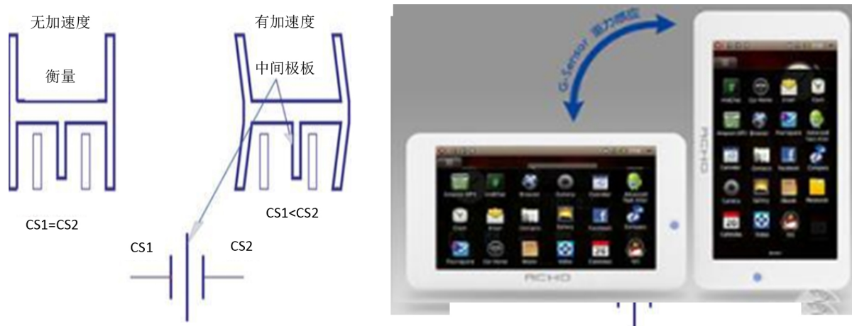
Figure 2. Schematic diagram of capacitive MEMS acceleration sensor and its application in smart phone
