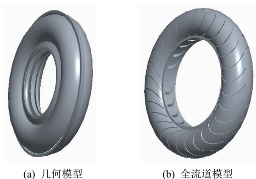
Figure 13. Parametric geometric and whole channel models of the torque converter
