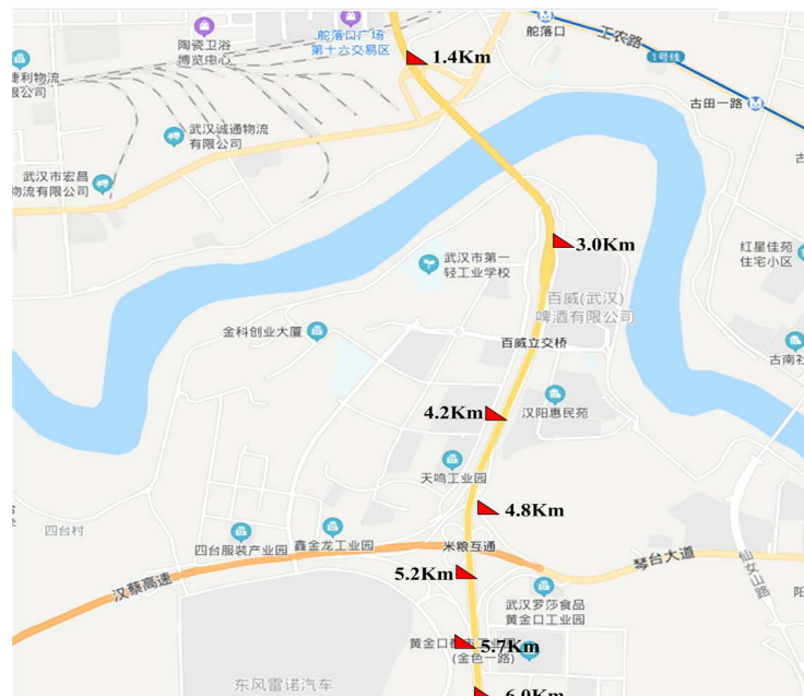
Figure 2. Layout of multi point distance measurement between LoRa terminal and LoRawan gateway
