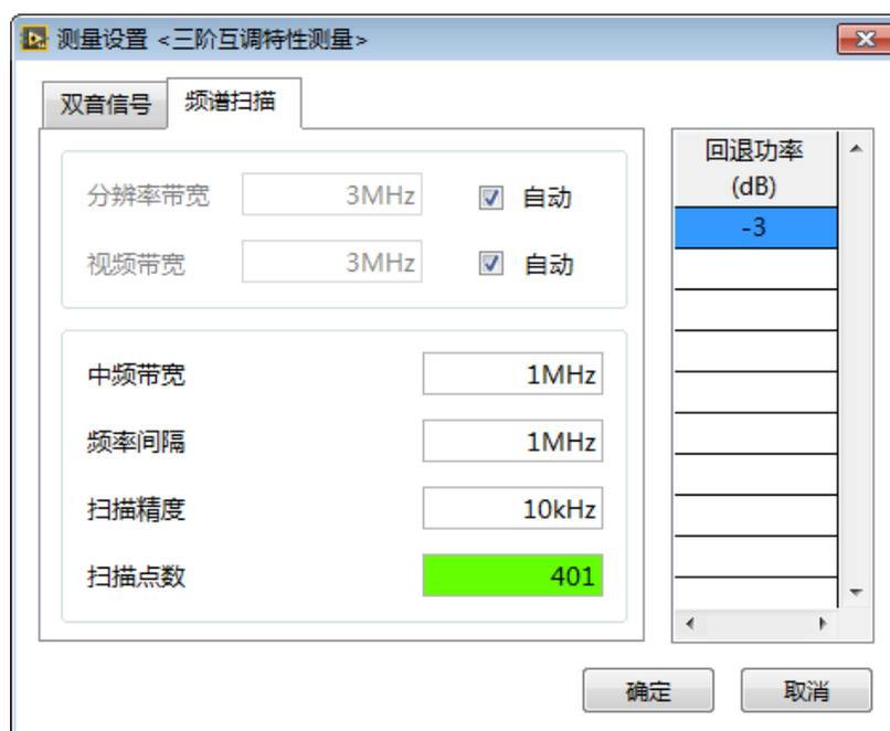
Figure 6. Setting for the third order intermodulation
