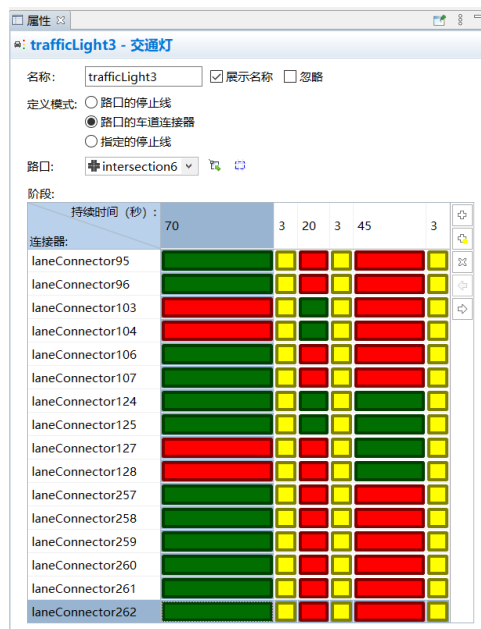
Figure 3. Basic attribute settings of TrafficLight 图 3. TrafficLight 基本属性设置
