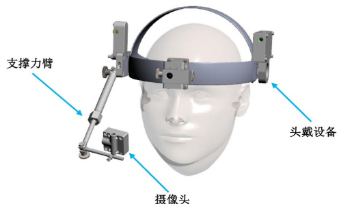
Figure 4. Schematic diagram of eye data acquisition equipment 图 4. 眼部数据采集设备示意图
