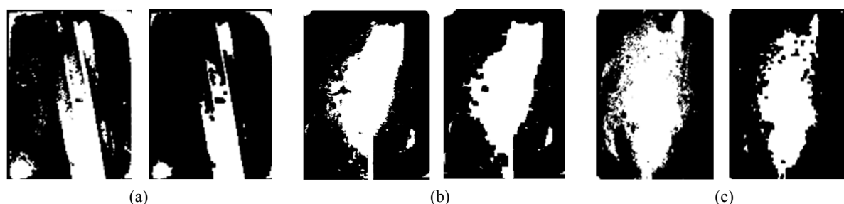
Figure 4. Binarization segmentation diagram and corrosion diagram. (a) Granular solder; (b) Standard solder; (c) Excess solder 图 4. 二值化分割图与腐蚀图。(a) 少锡; (b) 标准; (c) 多锡
