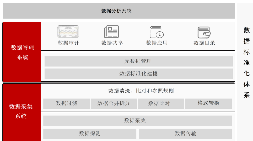
Figure 3. Functional architecture diagram of test big data comprehensive management platform 图 3. 试验大数据综合管理平台功能架构图
