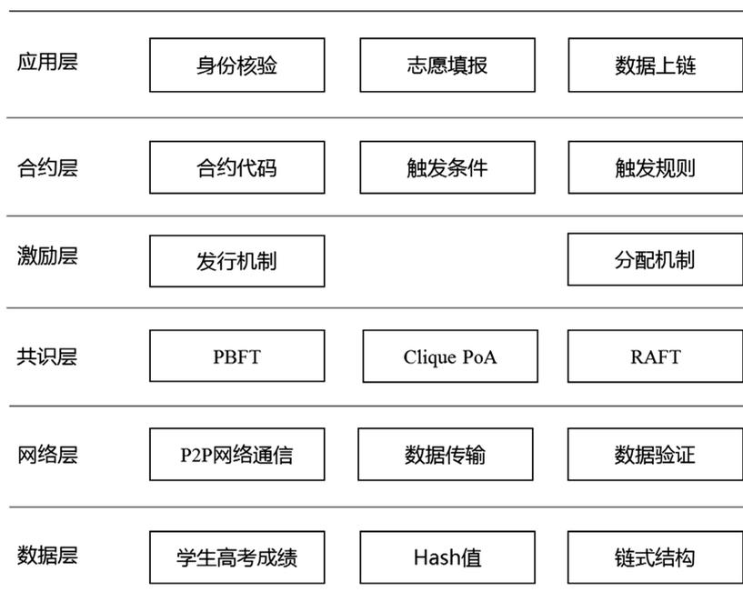
Figure 4. System underlying architecture
