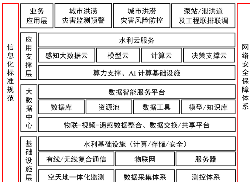
Figure 2. Overall architecture of the cloud platform
