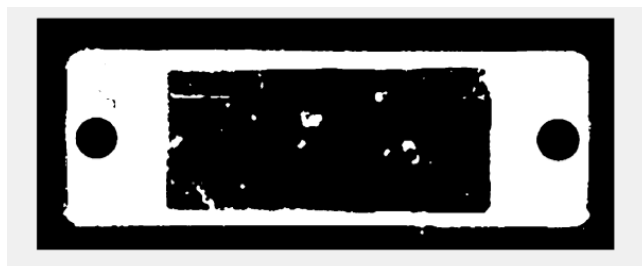
Figure 3. Image segmentation by maximum between-class variance 图 3. 最大类间方差法分割图像
