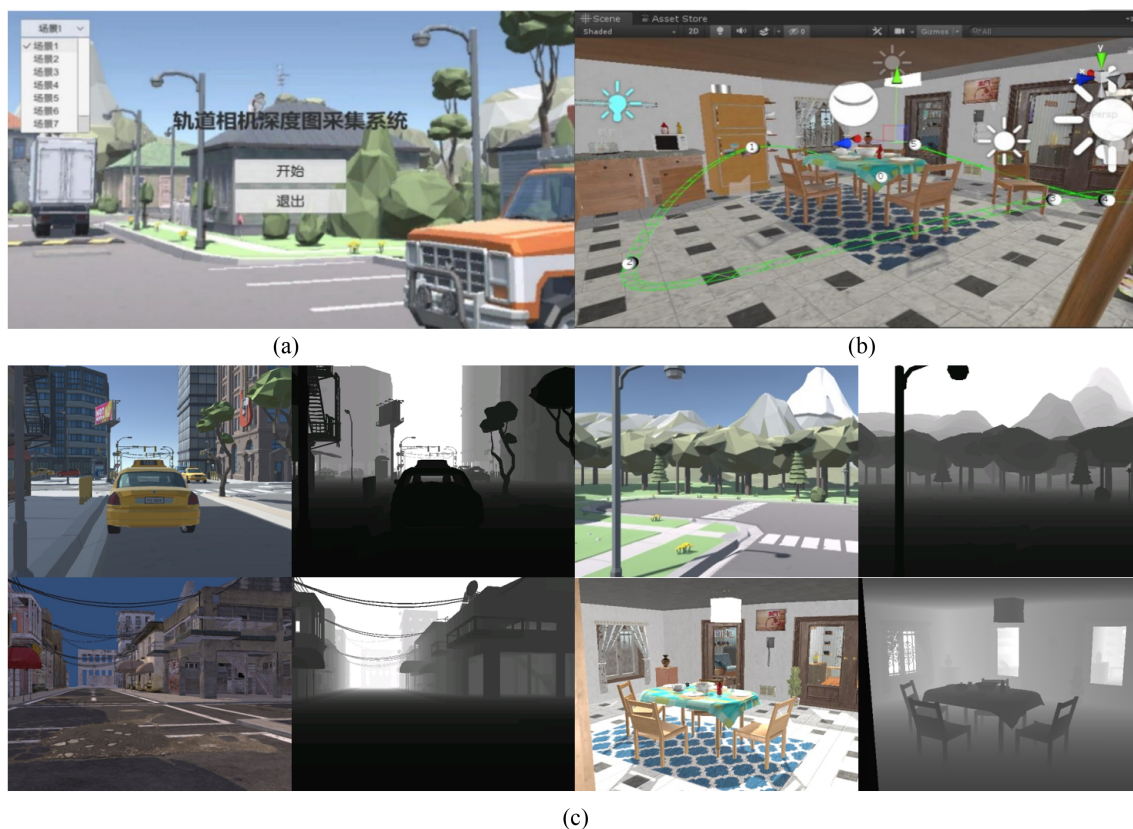
Figure 5. (a) The main interface of the track camera depth map acquisition system; (b) Example of indoor scene tracks; (c) Examples of a SU3D dataset: the first and third columns are the original image, and the second and fourth columns are the corresponding GT depth
