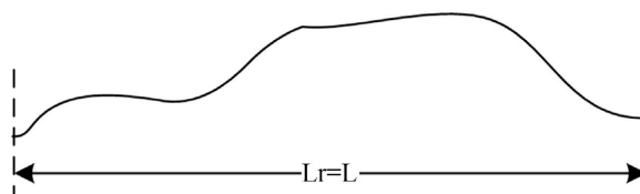
Figure 11. Diagram of crack sampling length over a long period 图 11. 裂缝取样长度过长时示意图
