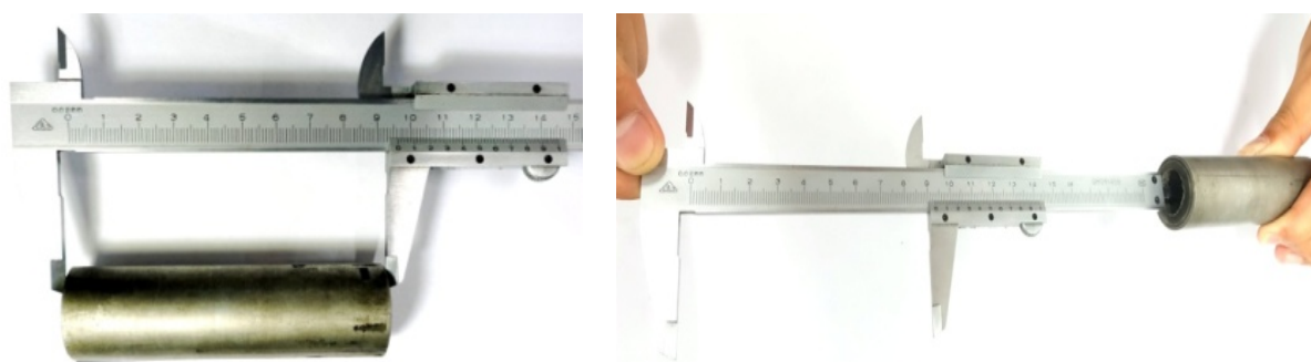
Figure 5. The machined hole with molybdenum-titanium-zirconium alloy by intelligent adaptive EDM
