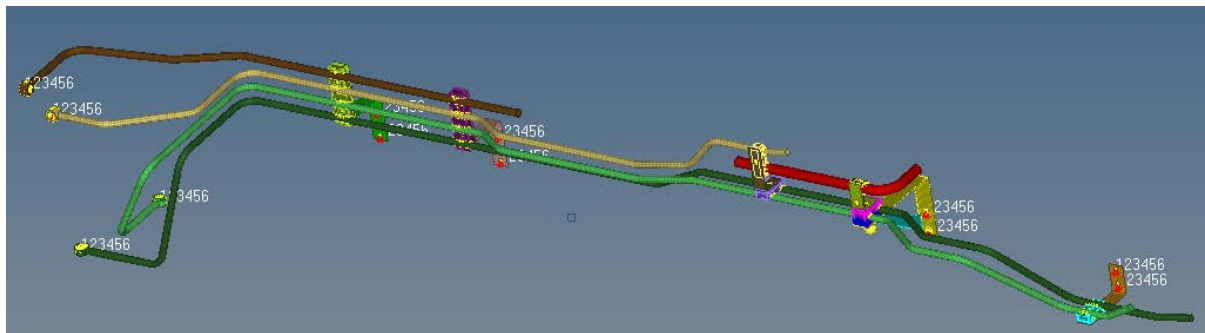
Figure 1. Layout of simplified finite element model for steering piping system
