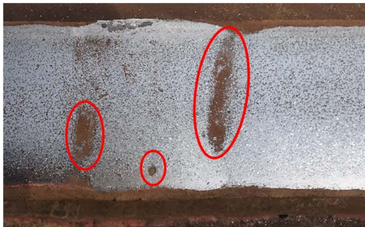
Figure 4. Figure of defects of the track tread (the white part is the contact position of the wheel and the track; the red circle is the track tread defect) 图 4. 轨道踏面的缺陷图(白色部位为车轮与轨道接触位置; 红圈为轨道踏面缺陷)
