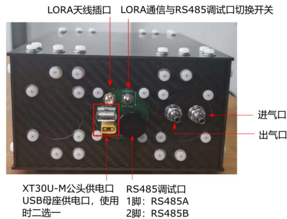
Figure 3. External interface of gas detection module 图 3. 气体检测模组外部接口
