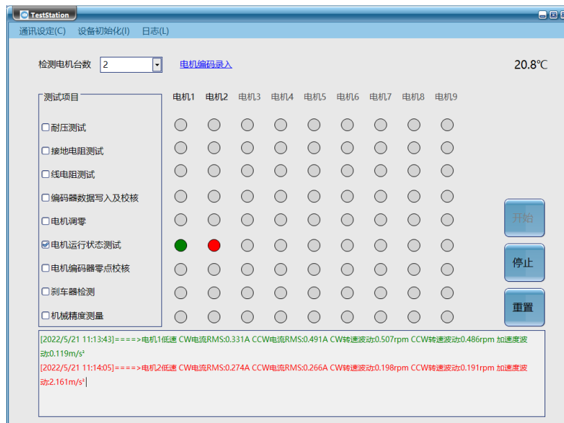
Figure 10. Motor running state test verification 图 10. 电机运行状态测试验证
