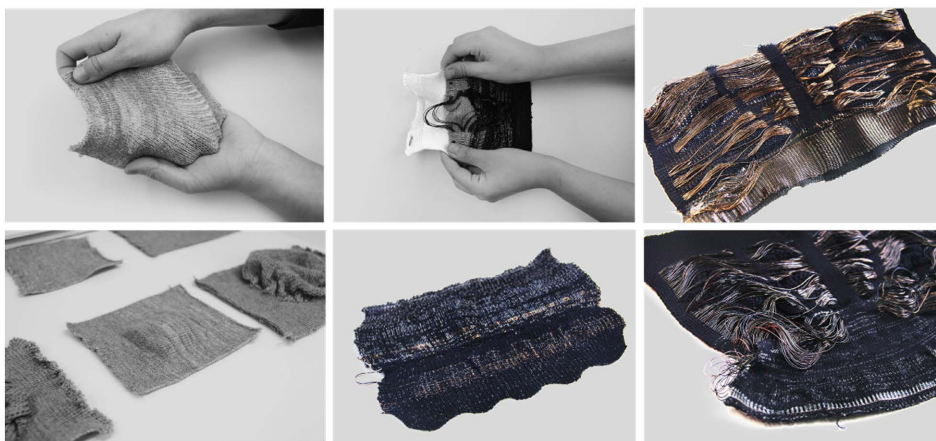
Figure 1. Material tests and textile structure experiments 图 1. 材料选择和纺织结构实验
