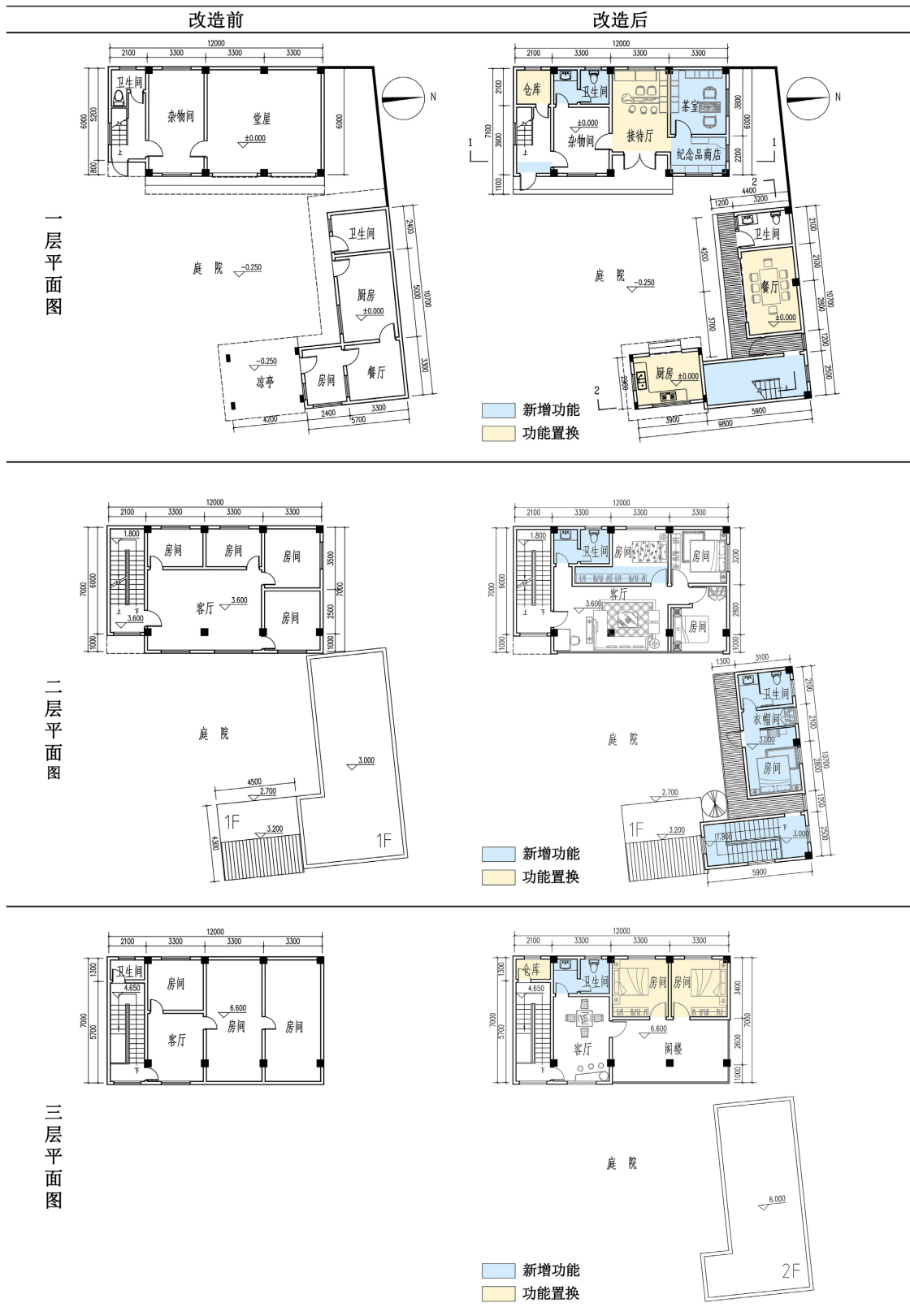
Figure 3. Comparative analysis of the floor plan before and after the renovation of the farmhouse 图3. 农宅改造前后平面图对比分析
