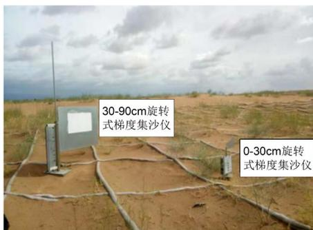
Figure 4. Rotary gradient sediment collector
