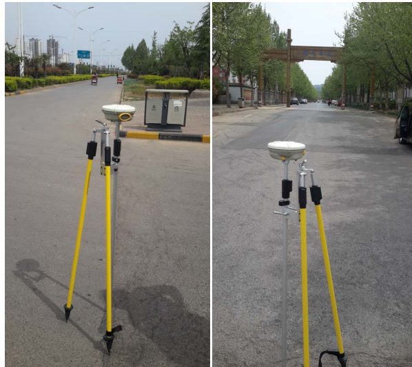
Figure 1. Photos of control point layout and measurement 图 1. 像控点布设和测量照片
