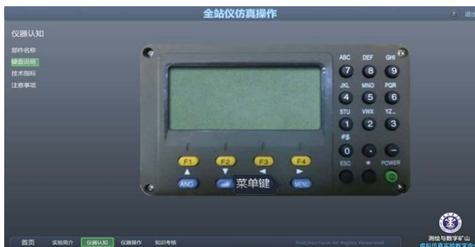
Figure 3. Total station keyboard simulation operation interface 图 3. 全站仪键盘模拟操作界面
