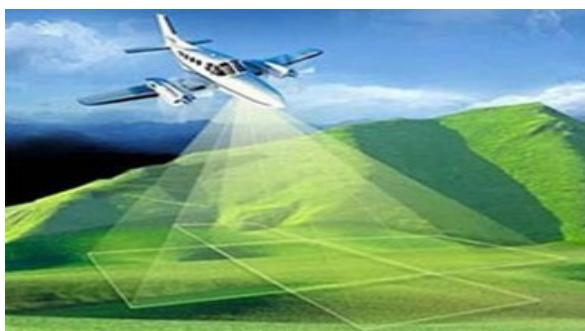
Figure 2. UAV oblique photography data acquisition system 图 2. 无人机倾斜摄影数据采集系统
