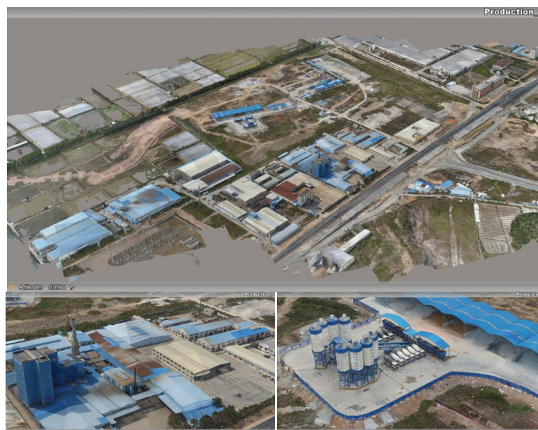
Figure 5. Overall and locally 3D real scene models of Sanjiang Interchange Area 图 5. 三江互通区整体及局部倾斜三维实景模型
