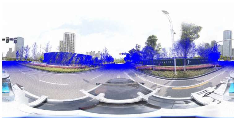
Figure 3. Illustration of the fusion of point clouds and panoramic images 图 3. 点云和全景影像的初始融合
