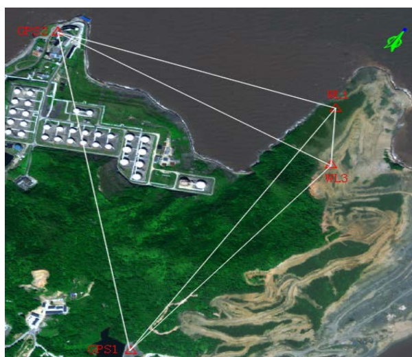
Figure 1. First level control network plan
