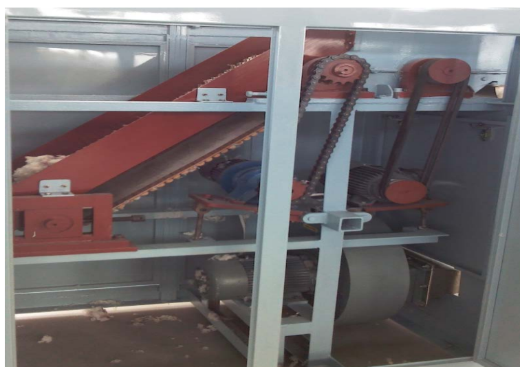
Figure 1. Lint-opening equipment in kind 图 1. 皮棉开松设备实物
