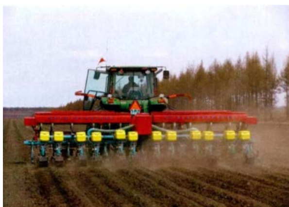
Figure 1. Fine variable fertilizer applicator with GPS [33] 图 1. 装备有 GPS 的精细变量施肥机[33]
