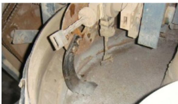
Figure 3. Schematic diagram of the installation of the bionic blade 图 3. 仿生刀安装示意图
