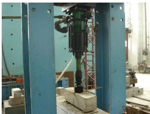
Figure 1. The fatigue experiment under the level of stress under the level of stress 图 1. 应力水平下的疲劳实验
