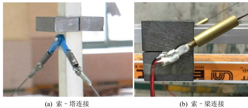
Figure 7. Connections of cables 图 7. 斜拉索的连接
