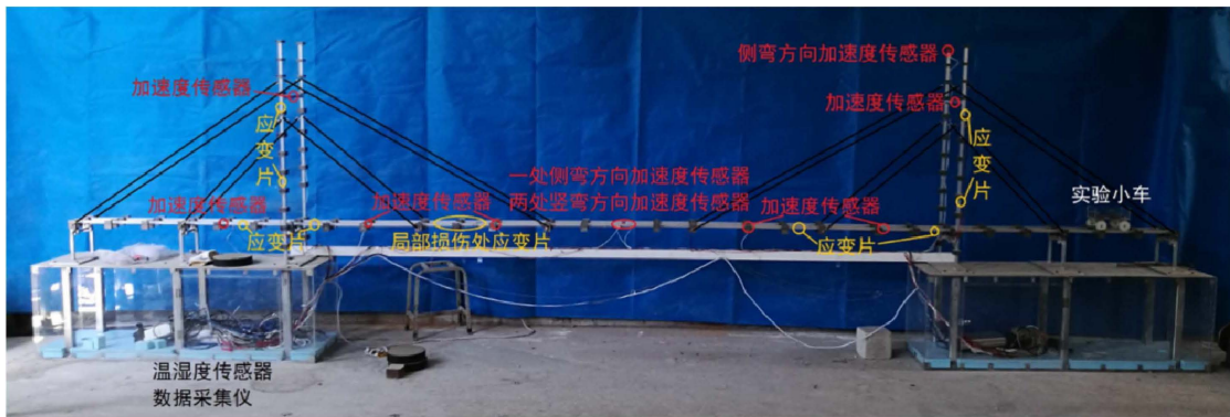
Figure 3. Scaled cable-stayed bridge demonstrative model 图 3. 缩尺模型图示
