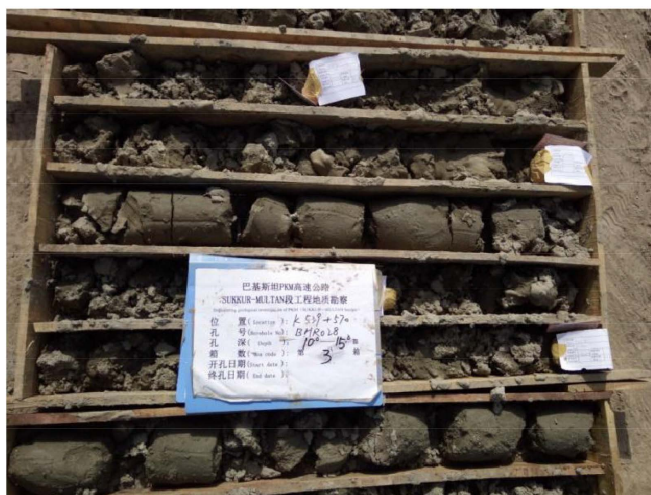
Figure 6. The SPT test sampling in drill holes 图 6. 钻孔 SPT 测试取样
