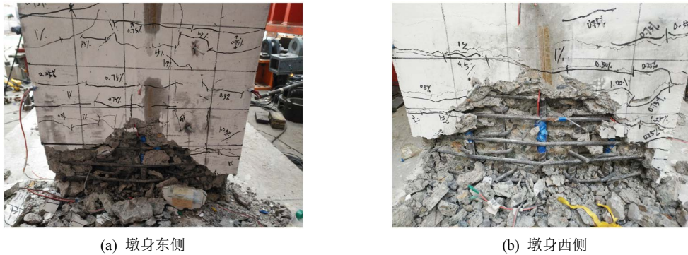
Figure 5. Failure modes of cast-in-situ pier specimen 图 5. 现浇桥墩试件破坏形态
