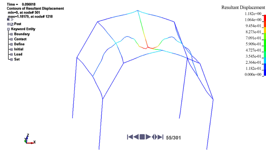
Figure 11. The diagram of maximum displacement of support rope 图 11. 支撑绳最大位移图
