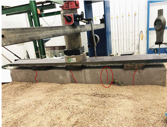
Figure 8. Failure diagram of 10 cm specimen 图 8. 10 cm 试件破坏图
