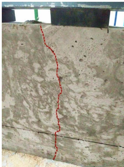
Figure 9. Failure diagram of 30 cm specimen 图 9. 30 cm 试件破坏图
